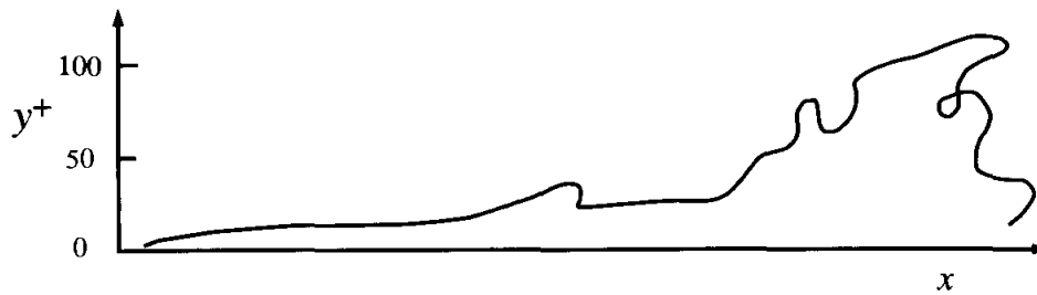
Fig. 7.40. A dye streak in a turbulent boundary layer showing the ejection of low-speed near-wall fluid. (From the experiment of Kline et al. (1967).)
